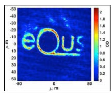
Ultracold atoms confined to a microscopically patterned potential. Areas of high optical/atomic density (OD) are indicated in the figure.
